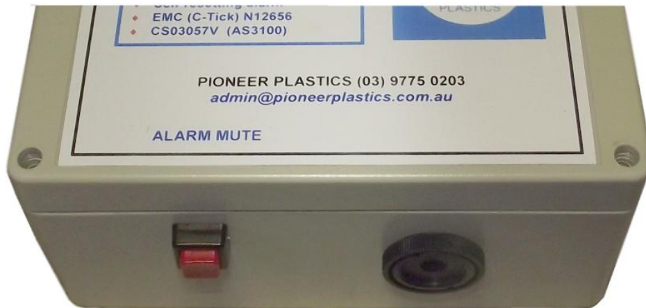
Bottom view showing the ALARM MUTE button and alert beeper
